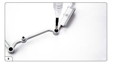
Take the Right Tie Rod and Center Link assembly. Locate the free eyelet at the end of the Center Link and align it with the eyelet on the end of the Left Tie Rod, as orientated in the picture. Connect the two parts with another MD06 screw, again only tightening so much that the parts are able to move freely.
